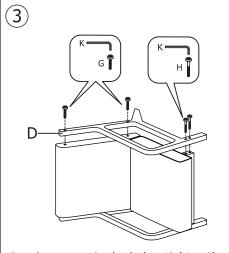
Put the screws in the holes, tighten the screws, but not too tight, 90% is ok.
