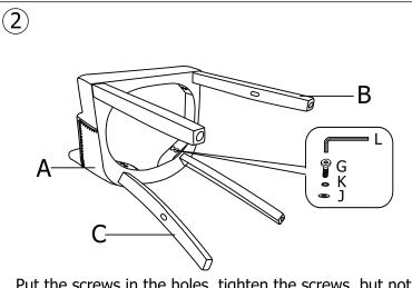
Put the screws in the holes, tighten the screws, but not too tight, 90% is ok.
